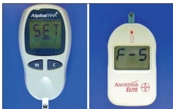
Figure 1: AlphaTRAK® (left) and Ascensia ELITE® (right) portable meter to measure blood glucose concentrations in cats.
