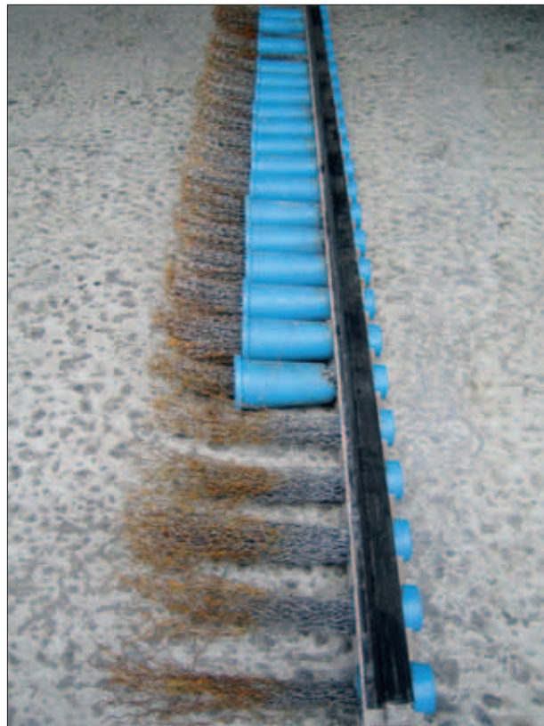
Figure 3: Wire brush attachment from runway cleaning machine.
