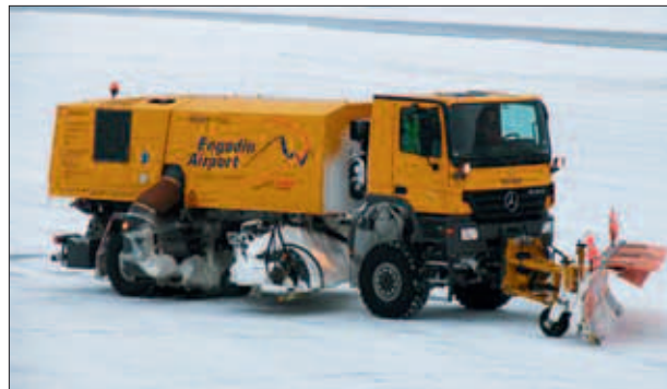
Figure 2: Runway cleaning machine with snow plough.
