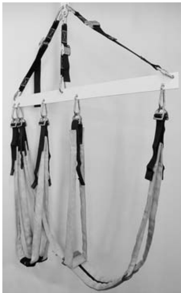
Figure 1: The UC Davis LAL consists of a counterbalance bar and two sling components made out of nylon straps.
