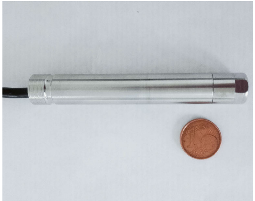
Figure 1: Opto-chemical oxygen sensor (TecMicro, Tecsense); the sensor is placed in the tip of the device and is immersed in the fluid for measurement
