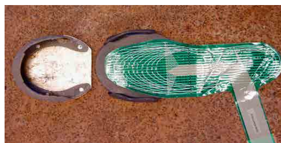
Fig. 1: Tekscan F-SCAN and the horseshoe system prepared for measuring the force of a kick.
