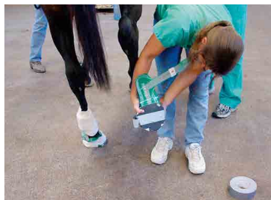
Fig. 2: The sensor and specialized shoe are attached to the sole of the foot.
